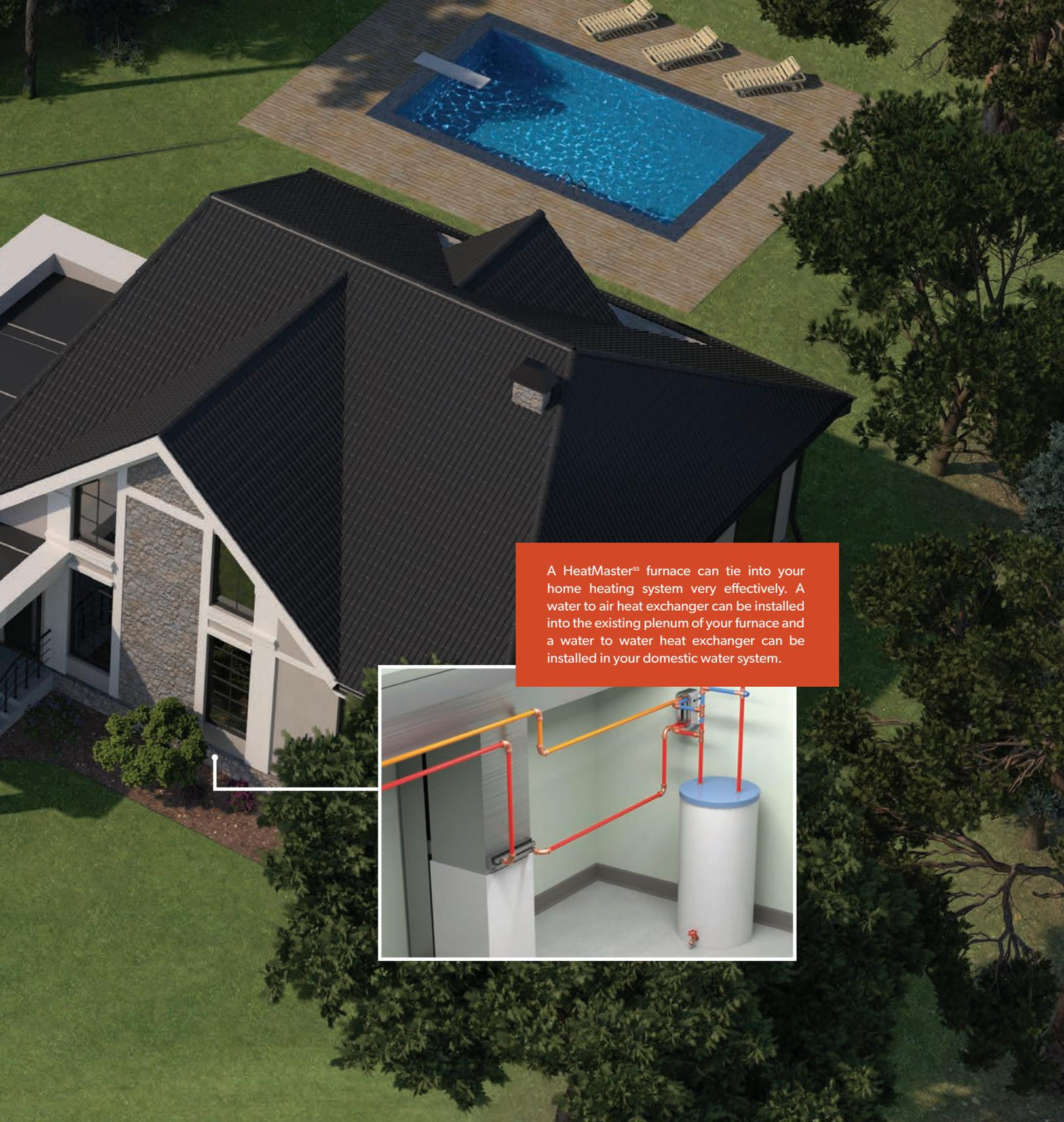
A HeatMaster<sup>®</sup> furnace can tie into your home heating system very effectively. A water to air heat exchanger can be installed into the existing plenum of your furnace and a water to water heat exchanger can be installed in your domestic water system.
